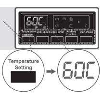
You can gradually decrease the washing water temperature between the maximum temperature and cold washing (--) by pressing washing water temperature adjustment button.
