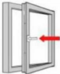
Turn the handle HORIZONTALLY : window opened
